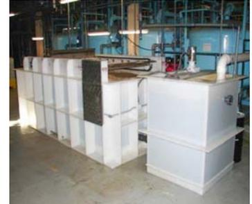
The recycle pressurization method is responsible for adequate loading of air bubbles into the system. High pressure (~100 psi) recirculation system supersaturates the water with air. When this water flows into the wastewater floatation tank micro-bubbles (~30  $\mu\text{m}$ ) form. The micro-bubbles adhere to waste particles and cause them to float to the surface where they are removed with a sludge flight system.
