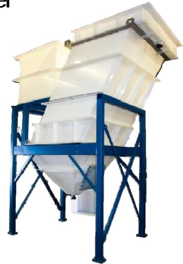
The outlet area utilizes removable type weir boxes with orifices to force uniform upward pressure over the entire plate area. Each plate section provides equalized flow to prevent channeling. The clarified water gravity flows from the top of the clarifier to the customers discharge point.
